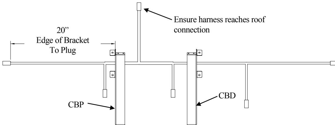
5. Fasten brackets CBD and CBP (with harness) to the roof. Do not fully tighten in order to allow movement of the brackets. Use fasteners from step 1.
