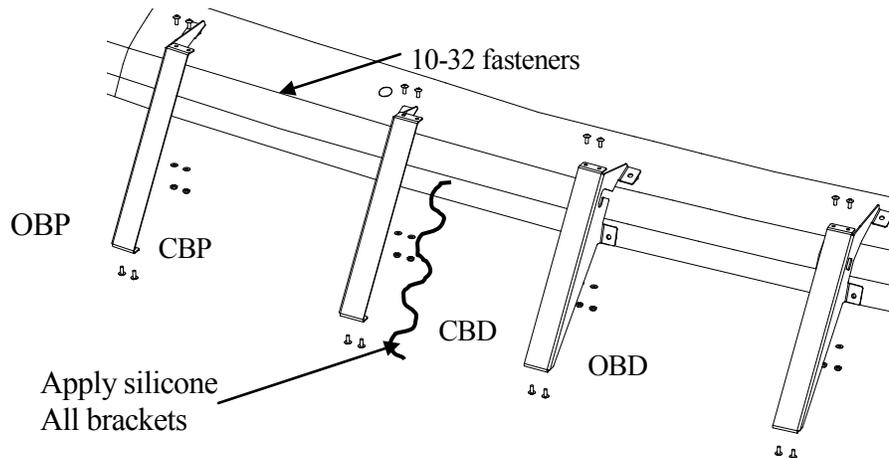
7. Apply silicone to the front face of all the brackets.
